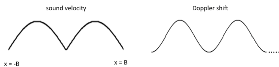
Figure 5. Sinusoidal Doppler FM from Accelerating Motion
